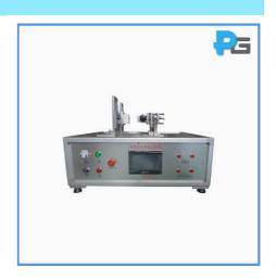
The life tester uses the cylinder as the power to drive the slide rail assembly with clamps to do reciprocating rectilinear movement, thereby completing the insertion and extraction of the plug and the socket. The operating frequency and switching time are controlled by PLC and LCD display.
