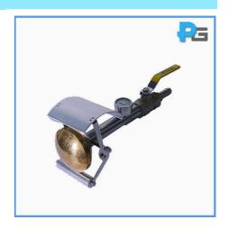
150kPa, and it should be kept constant during the test, the test duration is 1min/m² of the calculated surface of the enclosure and with a minimum duration of 5 min. For IPX4 test, the counterbalanced shield is removed from the spray nozzle and the enclosure is sprayed from all practicable directions, the rate of water flow and the spraying time per unit area are same as IPX3 test.
