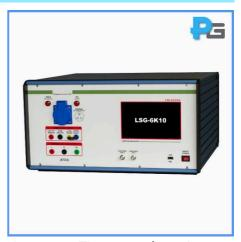
The lightning surge generator can generates both 1.2/50, 8/20 µs combination wave. The test voltage is up to 6KV, user can choose and define the test levels. The parameters of waveform for surge voltage and waveform for surge current is strictly meet the standard requirements of IEC61000-4-5. It is built in a 300V/10A coupling and decoupling network.
