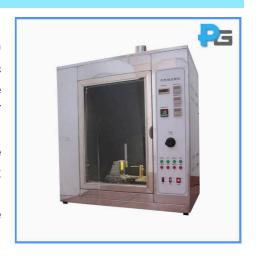
Glow wire testing is an electrical safety test designed to evaluate the flame resistant properties of plastic materials used in electrical devices. Its purpose is to protect against the risk of fire from overheated or electrically energised parts which may cause the plastic material to ignite. This may occur in normal use, under reasonable abnormal use, malfunction or failure of the product. The glow wire simulates an over-heated part which then comes into contact with plastic materials.
