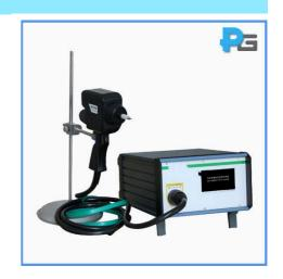
The ESD generator is consisted by ESD generator, ESD gun and two electrodes (cone sharp electrode is for contact discharge, and ball sharp electrode is for air discharge), the parameters of rising time, peak current and current at 30ns and 60ns are strictly meet the requirement of IEC61000-4-2.
