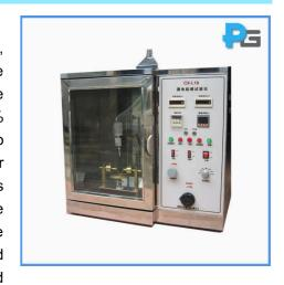
Proof Tracking Index (PTI): the voltage value of the material subjected to 50 drops of electrolyte without electrical tracking, the unit is volt.
