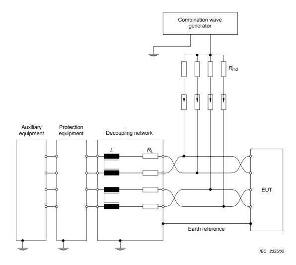
Calculation of  $R_{m2}$  when using CWG (1,2/50  $\mu$ s generator)
