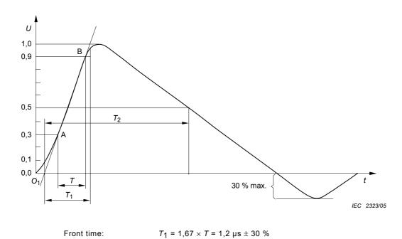
NOTE The open circuit voltage waveform at the output of the coupling/decoupling network may have a considerable undershoot, in principle as the curve shown in Figure 3.
