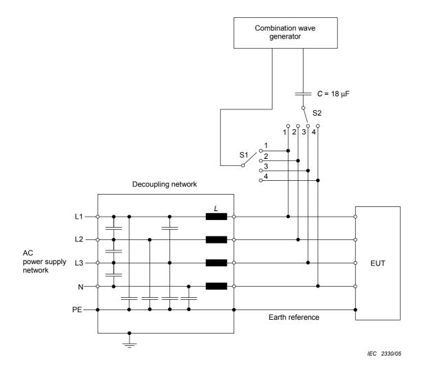
Figure 9 – Example of test setup for capacitive coupling on a.c. lines (3 phases); line L3 to line L1 coupling (according to 7.2)
