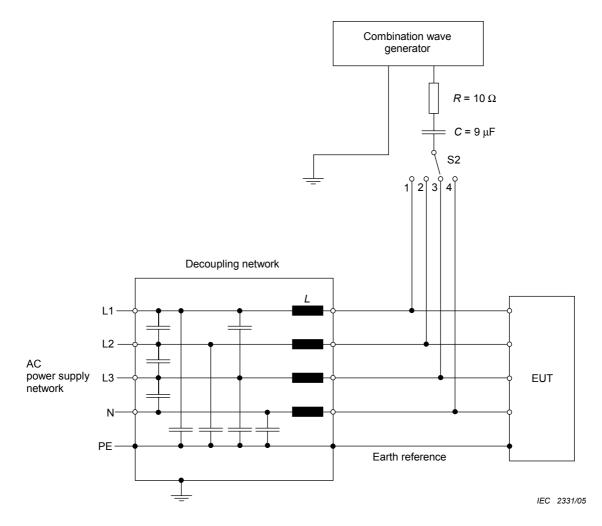
Switch S2 is used to select individual lines for test.
