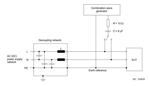
Figure 8 – Example of test setup for capacitive coupling on a.c./d.c. lines; line-to-ground coupling (according to 7.2)
