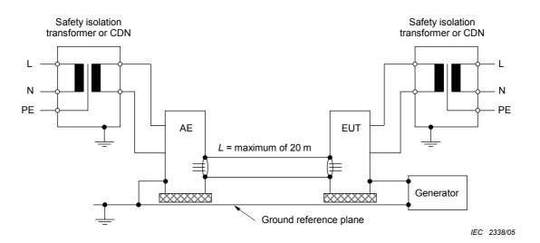
NOTE 1 It is permissible for the power to the EUT and/or the AE to be provided via a decoupling network as shown in e.g. Figure 7, rather than via the isolation transformer shown. In this case, the EUT's protective earth connection should be left open circuit.
