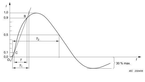
Front time:  $T_1 = 1,25 \times T = 8 \ \mu s \pm 20 \ \%$ Time to half-value:  $T_2 = 20 \ \mu s \pm 20 \ \%$
