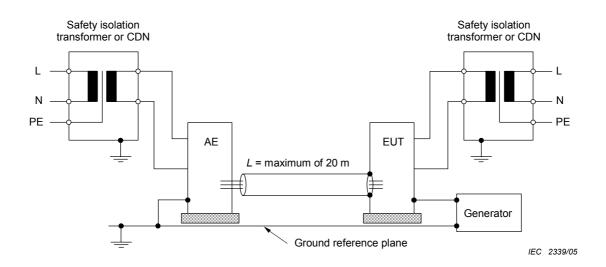
NOTE 1 It is permissible for the power to the EUT and/or the AE to be provided via a decoupling network as shown in, for example Figure 7, rather than via the isolation transformer shown. In this case, the EUT's protective earth connection should be left open circuit.
